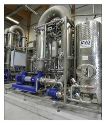
Photo 2: Ultrafiltration unit (Photo: SFPI)
